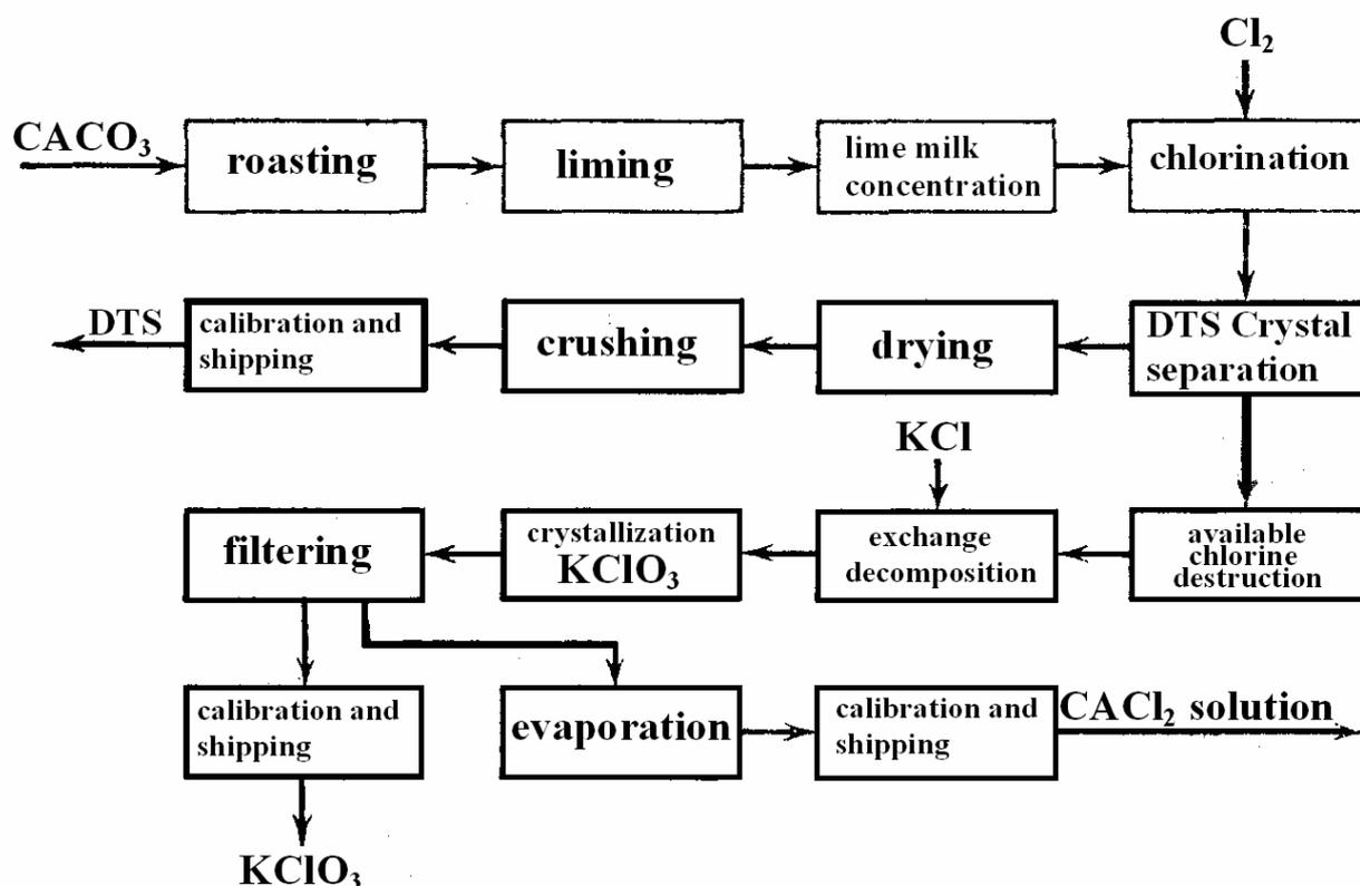
The product (hydrate) which crystallizes during the evaporation initially contains six molecules of water. Then as a result of calcinations, water gradually vanishes from the product and at temperature of 260°C waterless  $\text{CaCl}_2$  is produced as solid porous paste.
