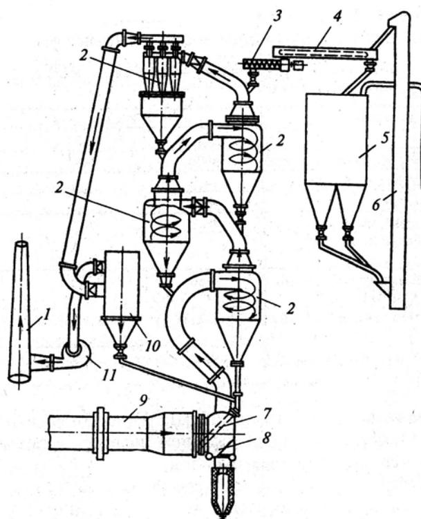
1 – chimney; 2 – cyclone heat-exchangers; 3 – screw feeder; 4 – scraping conveyer; 5 – feed hopper for ground resources; 6 – ladle elevator; 7 – discharge hopper; 8 – adapter; 9 – rotary kiln; 10 – dust collectors; 11 - smoke exhauster
