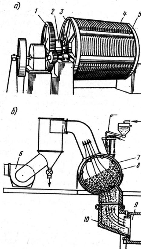
*a* – slime concentrator; *b* – scheme of connection of slime concentrator with loading end of rotary kiln
