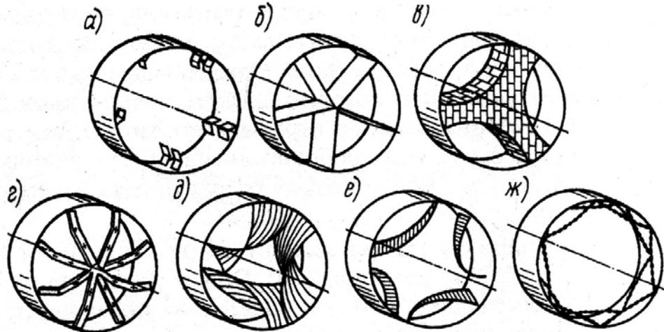
a – interspersing (lifting) vanes; б, в – cellular; г – link; д – arc; е – cycloid; ж – chain
