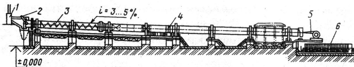
1 – smoke exhauster; 2 – feeder for feeding slime; 3 – drum; 4 – drive; 5 – ventilator with burner nozzle for blowing of fuel; 6 – grate cooler
