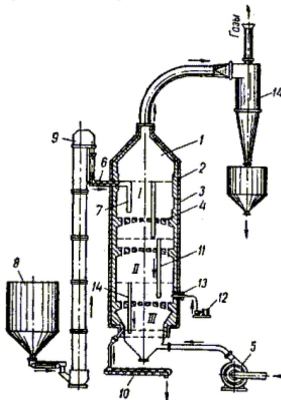
1 – reactor; 2 – refractory brick; 3 – steel case; 4 – grate roof; 5 – ventilator; 6 – screw feed ; 7 – limestone feed pipe; 8 – bunker for grinding resources; 9 – elevator; 10 – screw for drawing lime; 11 – pipes for transferring material from upper to lower zones; 12 – pump for fuel oil feed; 13 – burner nozzles; 14 – cyclone for cleaning gases of dust
