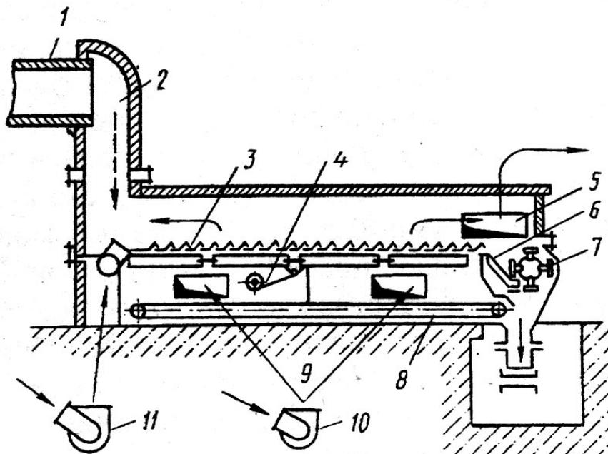
1 – rotary kiln; 2 – takeup shaft; 3 – fire grate; 4 – drive; 5 – window for discharge of surplus exhausted air to atmosphere; 6 – screen; 7 – hammer crusher; 8 – scraping conveyer; 9 – windows for general blast; 10 – ventilator of general blast; 11 – ventilator of "overgrate blast"
